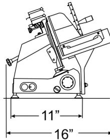
Our slicers have anodized aluminum alloy bodies. The high carbon steel blades are hard chromed, with a hollow ground taper for extended sharpening and blade life. These belt driven machines offer exceptional cutting consistency and durability. The carriage moves smoothly on ball bearings allowing effortless cutting of deli meats and vegetables. Easy to disassemble for quick cleaning. Perfect for low volume operations. Made in Italy.
